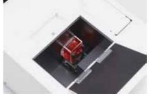
Transmittance Measurement: The CM-3600A/CM-3610A employs the d:0° geometry (diffuse illumination, 0° viewing), which conforms to ISO, CIE, ASTM, and DIN standards.
